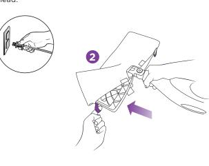
**2** Remove the micro-fiber cleaning pocket by releasing the quick fasteners and using the lavender loop on the side of the pocket, avoiding contact with the hot pocket or dirt. Then empty the water tank.
